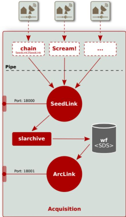
**SeedLink** collects waveform data from stations through plugins. Many plugins for various digitizers are available. **SeedLink** is a TCP server and delivers TCP data streams to remote clients on port 18000 (configurable).
