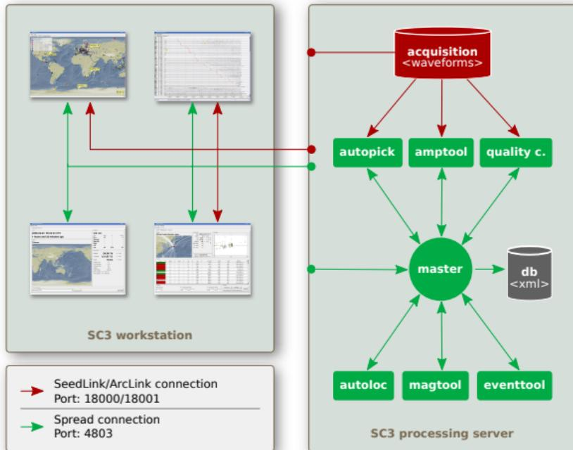
Automatic and interactive system each running on a dedicated computer. Both systems are connected to the same messaging and waveform server.
